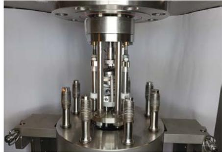
Fig. 1: Novel high pressure tribometer to investigate friction and wear of dry metal contacts in volatile lubricant environments.
