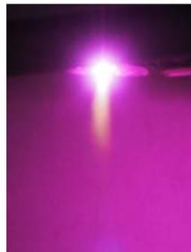
Fig. 2: Image of the water damp arc plasma with afterglow.
