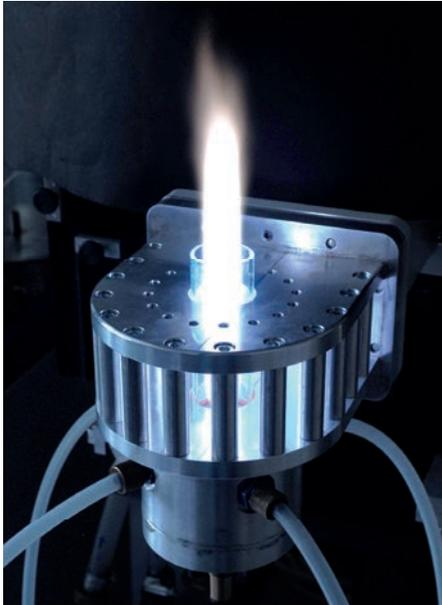
Fig. 1: Plasma torch fed by pressured air with four tangential inlets, here without the sampling apparatus for NO<sub>x</sub> detection.
