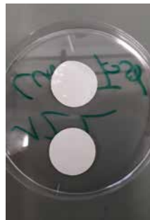
Fig. 2: Dip-coated and cross-linked hydrogel film on a membrane carrier foil.
