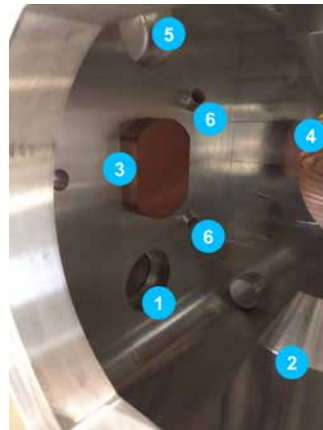
Fig. 2: Half of diplexer interior, looking through the hole for the other main resonator mirror: 1) input port, 2) matching mirror, 3) grating mirror for coupling into the resonator, 4) resonator main mirror, 5) non-resonant output port, 6) diagnostic horns for power measurements; the resonant output (not visible) is opposite the non-resonant port.
