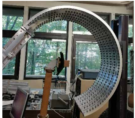
Fig. 2: Field measurement of the bent antenna.
