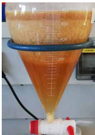
Fig. 1: Dewatering of the MEL containing culture broth by addition of chaotropic salts.
