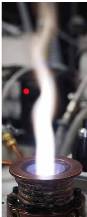
Fig. 1: Picture of the effluent free jet of a microwave air plasma at 1 kW microwave power and 20 slm air flow.
