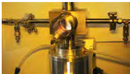
Fig. 1: Tubular reactor with a ceramic capillary inside. Argon flows from the left side through the capillary and the oxygen was measured with a \text{ZrO}_2 detector.
