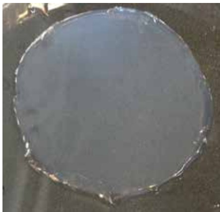
Fig. 1: Calcium alginate/polyacrylamide double network hydrogel.
