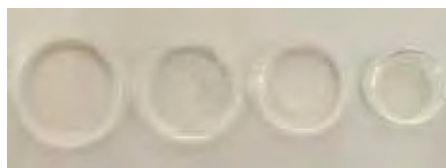
Fig. 2: Step growth network hydrogels prepared with different amounts of cross-links changing their swelling behavior. From left to right: 80%, 60%, 40% and 20% cross-linking.
