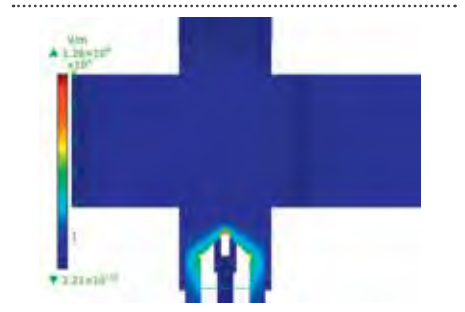
Fig. 2: Simulation of the electric field distribution inside the resonator. The electric field reaches up to 1.26 \cdot 10^6 V/m at the nozzle tip, if the tip is located 8 mm below the resonator base.
