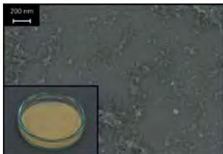
Fig. 1: SEM-picture of prepared Chitosan nanoparticles. Lower left corner: raw low molecular weight chitosan powder.
