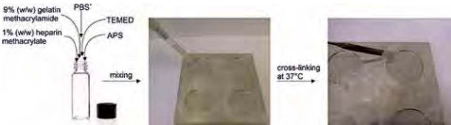
Fig. 1: Hydrogel preparation via thermal-redox initiated cross-linking of methacryl-modified gelatin and methacrylated heparin.
