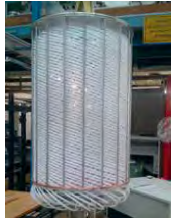
Fig. 1: 2-MW/CW load, with the outer shells removed, showing the twisted double layer of Teflon hoses with the conical reflector behind, and the water manifold on the right.
